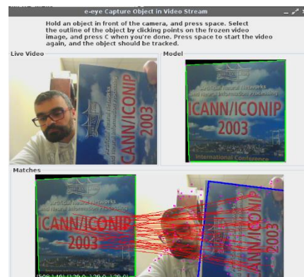
Fig. 11. Book object is found with the cross direction as original object in Matches frame
